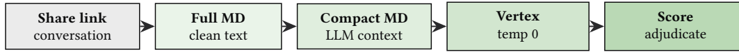
Figure 1. Evidence flow: conversation link to full Markdown, compact Markdown, Vertex extraction at temperature 0, deterministic aggregation, site-health join, then targeted adjudication/rescue for suspicious rows.
